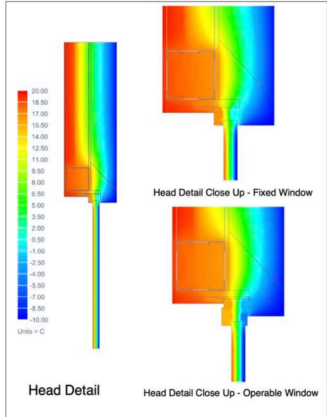
*Figure 1: Humber College Building NX window transition thermal modeling demonstrates the impact of thermal bridging control.*
