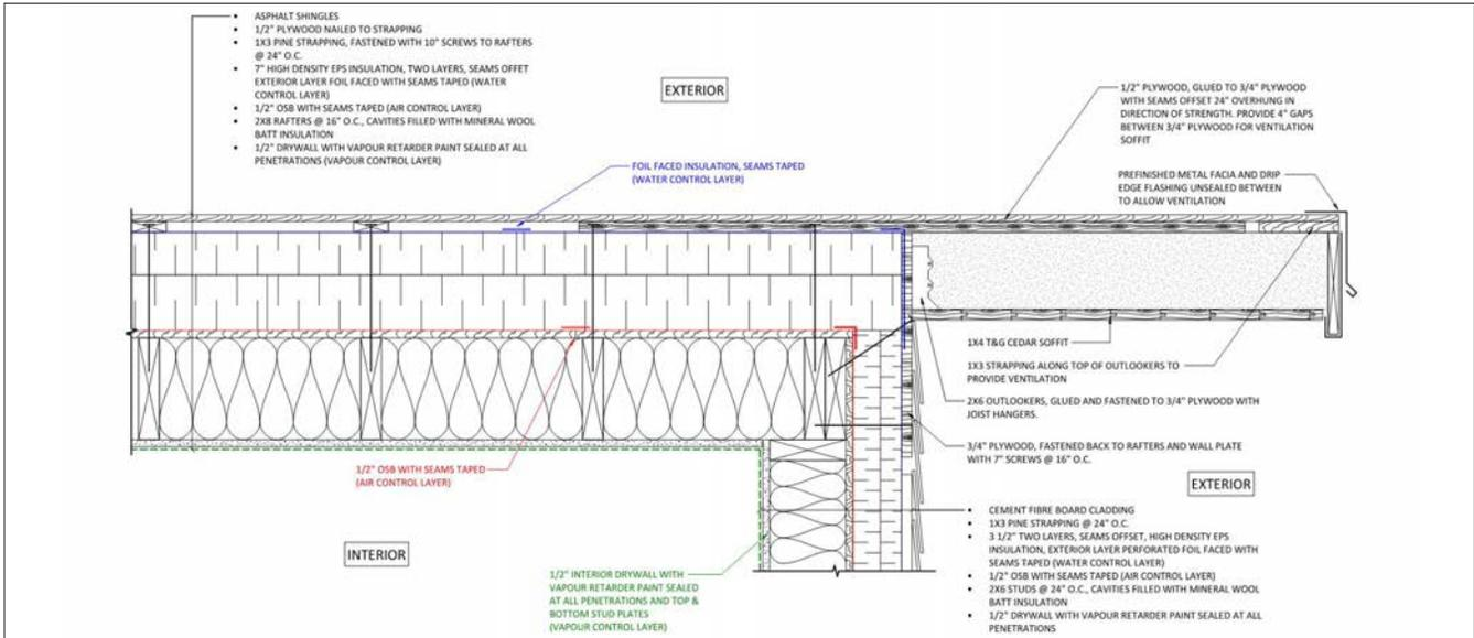
Figure 2: Wall-to-roof interface detail; note the continuous control layers and the exterior insulation that wraps continuously from the roof to the wall.
