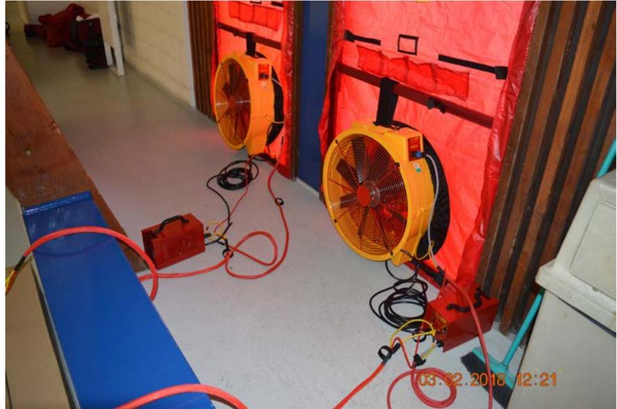
*Two blower door fans used for testing the building's air barrier performance.*
