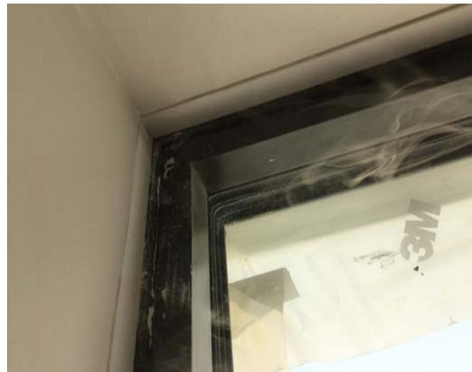
*Interior view of smoke infiltration during testing.*
