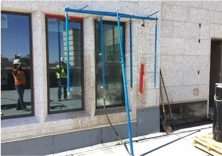
Exterior view of water testing a window assembly.
