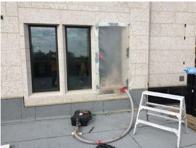
*Exterior view of smoke testing a window assembly to identify gaps in the air barrier.*
