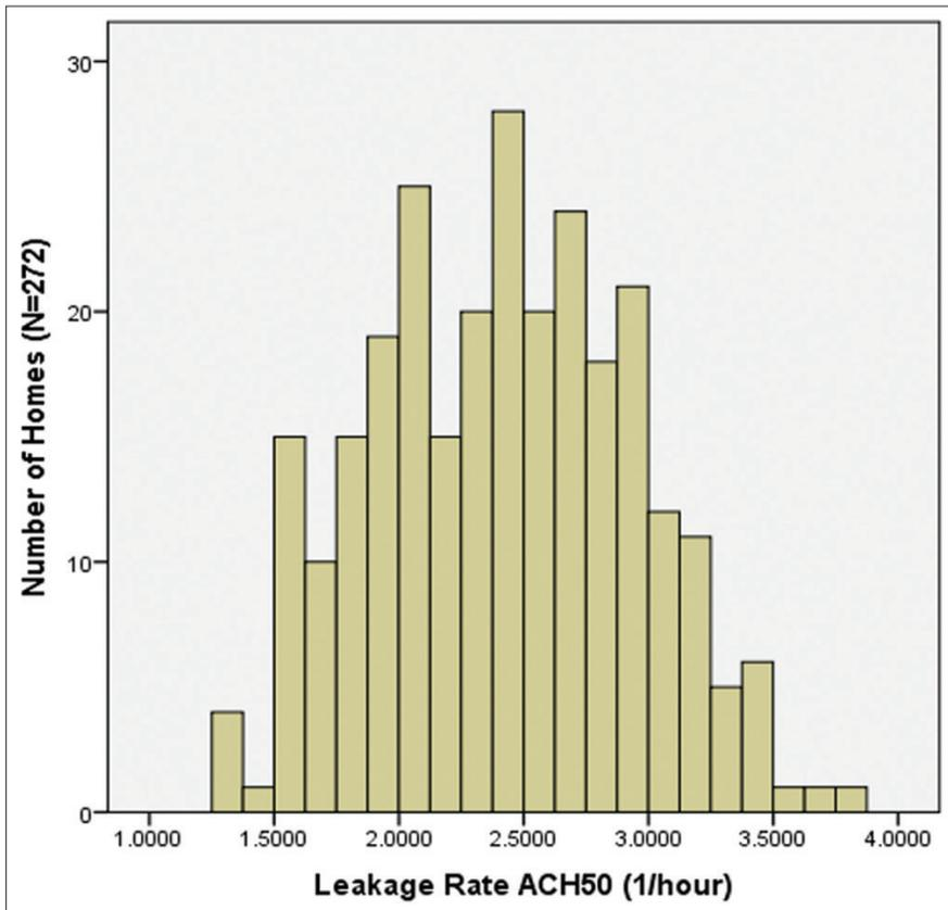
Figure 3. Distribution of airtightness subset used in modelling.
