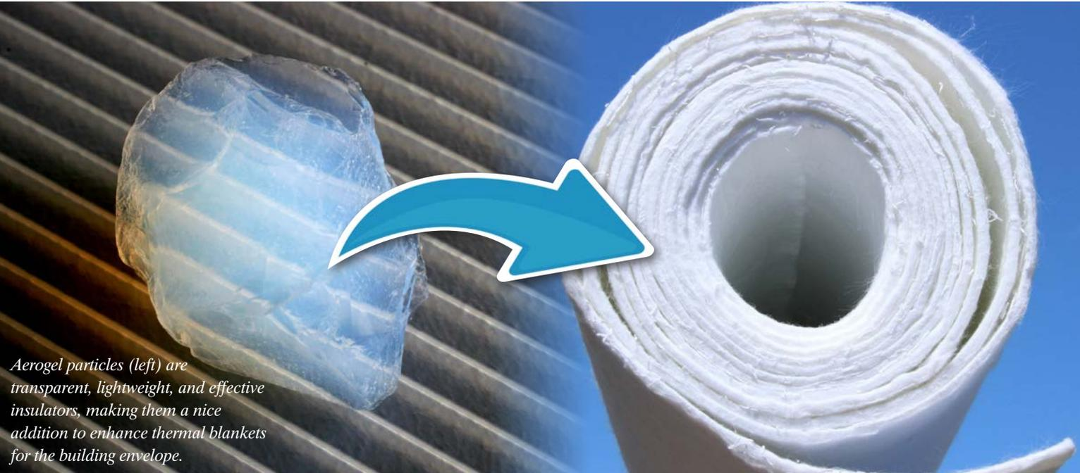
*Aerogel particles (left) are transparent, lightweight, and effective insulators, making them a nice addition to enhance thermal blankets for the building envelope.*
