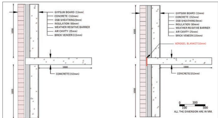
*Figure 1. Wall and floor connection with concrete structure (standard on the left, improved on the right).*
