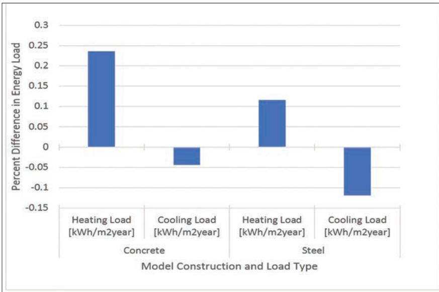
Figure 2. Per cent difference between energy loads for the base case model and improved model with aerogel blankets at thermal bridges.
