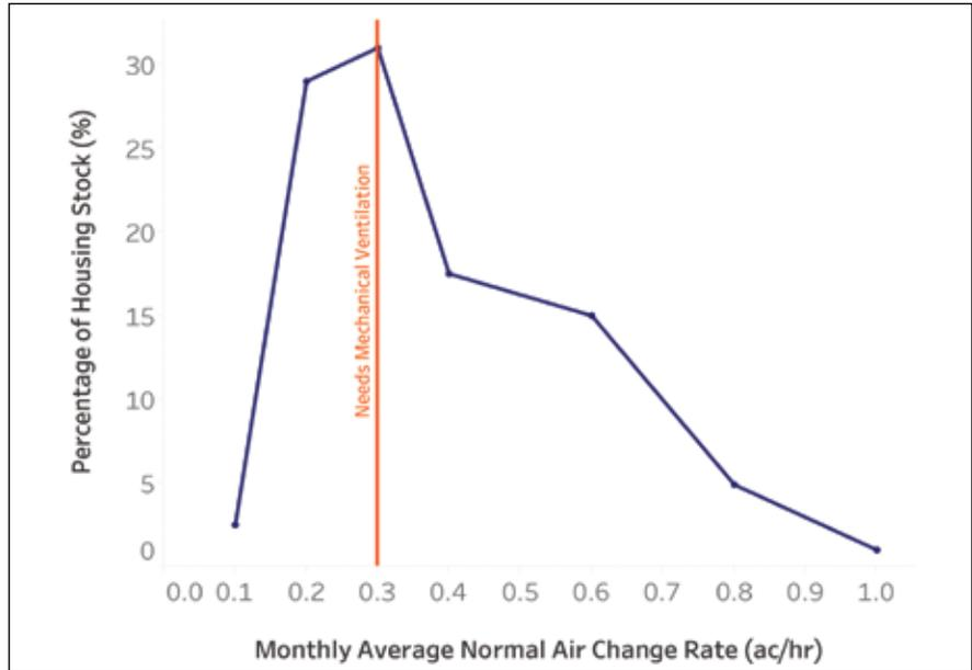
Figure 3. More than 62 per cent of stock is below the recommended normal air change rate of 0.3 and needs mechanical ventilation.<sup>6</sup>
