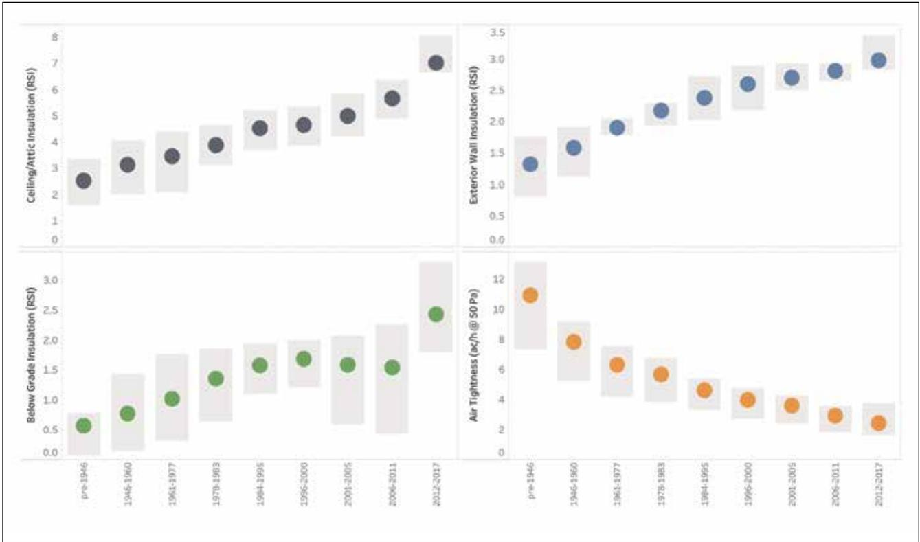
Figure 2. Envelope insulation levels (effective thermal insulation value in  $m^2K/W$ ) and average air-tightness of dwellings.<sup>4</sup>
