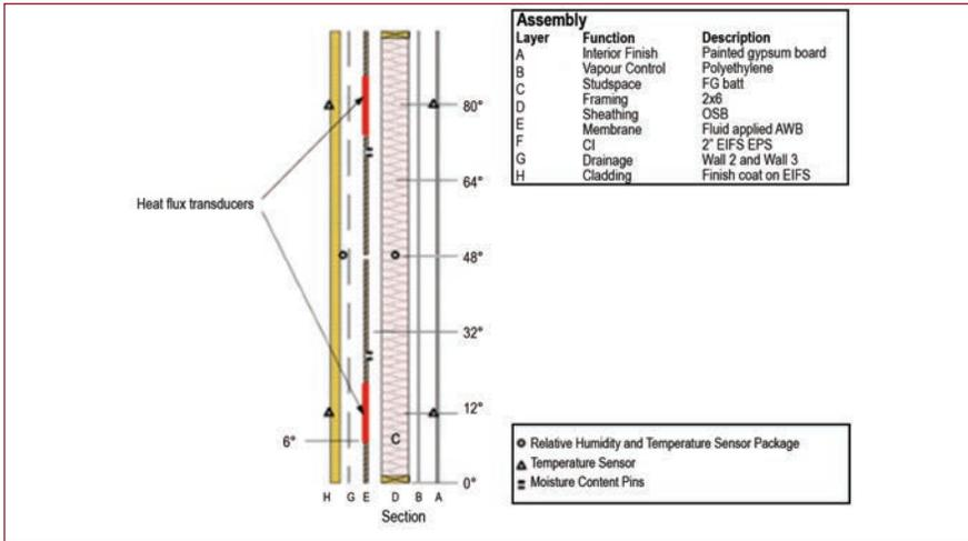
Figure 3. Field-tested wall assembly.
