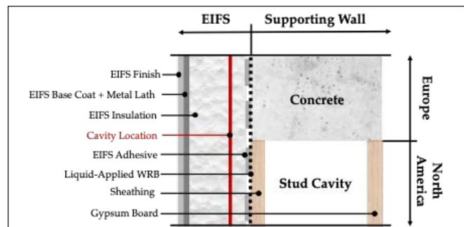
Figure 2. Typical EIFS construction in North America and Western Europe.
