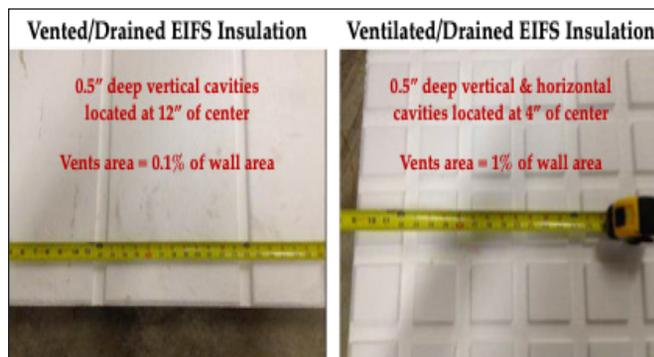
Figure 1. Vented vs. ventilated EIFS.
