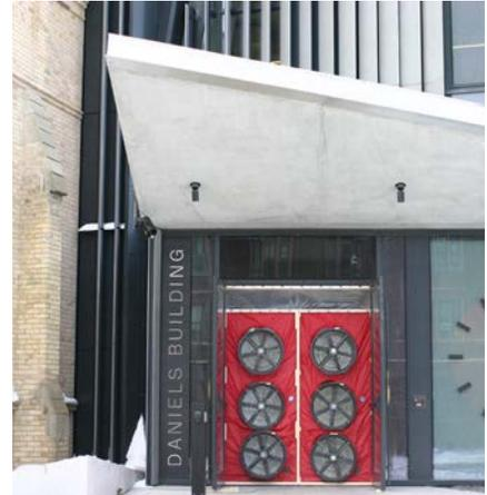
*The University of Toronto's Daniels Building's 1875 envelope was leaking three times more than the modern addition.*
