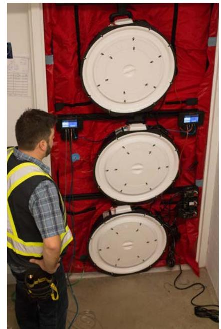
The University of Toronto's Daniels Building required 12 blower door fans to employ a guarded airtightness testing technique.
