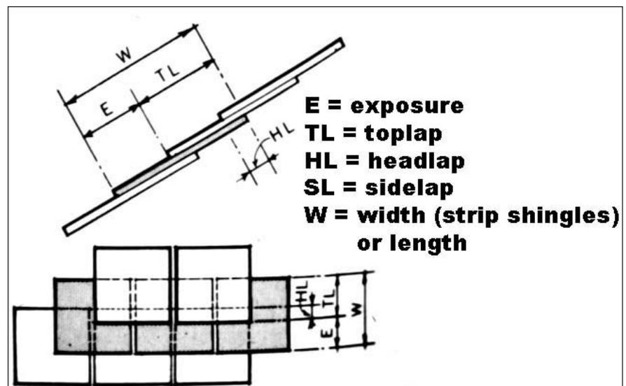
A diagram of the typical geometry of roof shingles.
