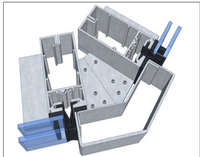
Figure 3. Ineffective fasteners at the corner mullion.
