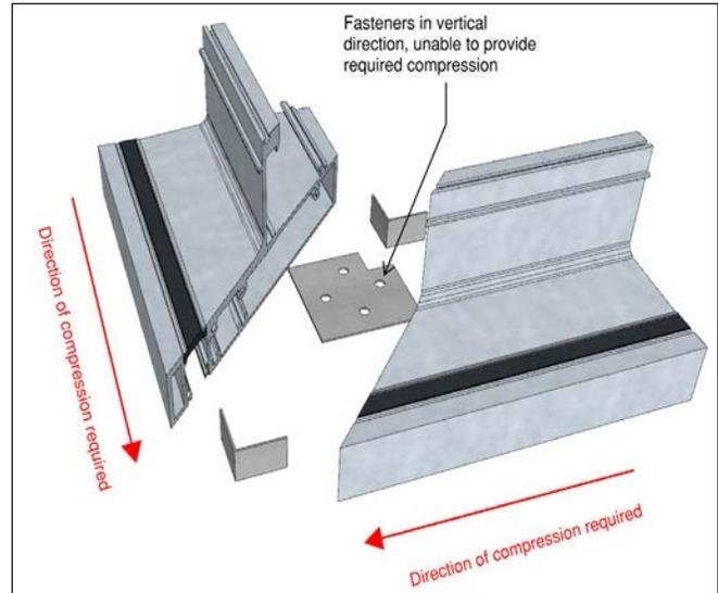
Figure 2. A standard corner detail. Note the four split mullions. Note, some fasteners, extrusions, and gaskets have been omitted.
