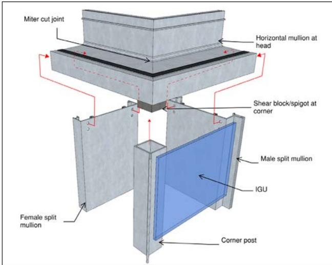
Figure 1. A conceptual model of an outside corner mullion using a corner post. Note, some fasteners, extrusions, and gaskets have been omitted.
